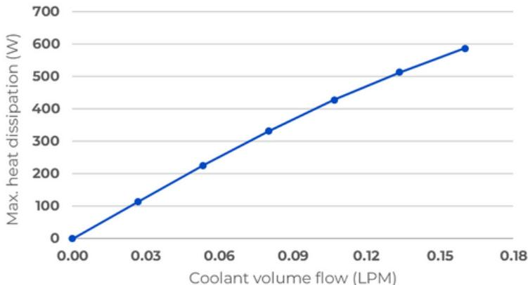
\*Heat dissipation considering 100°C fixed coil-former temperature.
