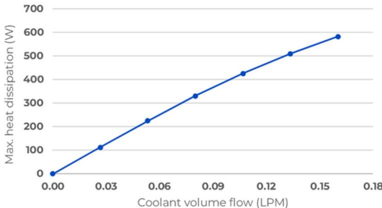
\*Heat dissipation considering 100°C fixed coil-former temperature.
