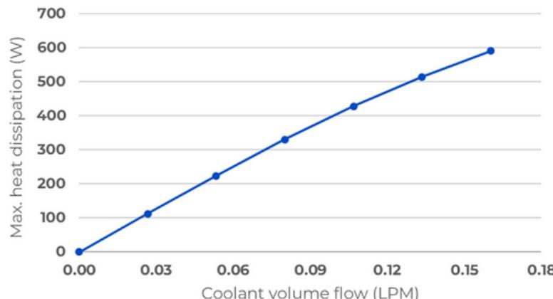
\*Heat dissipation considering 100°C fixed coil-former temperature.
