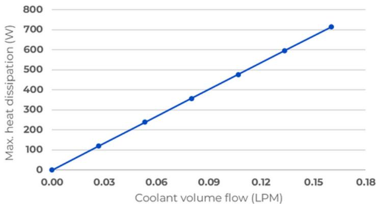
\*Heat dissipation considering 100°C fixed coil-former temperature.
