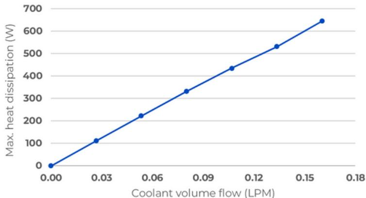
\*Heat dissipation considering 100°C fixed coil-former temperature.
