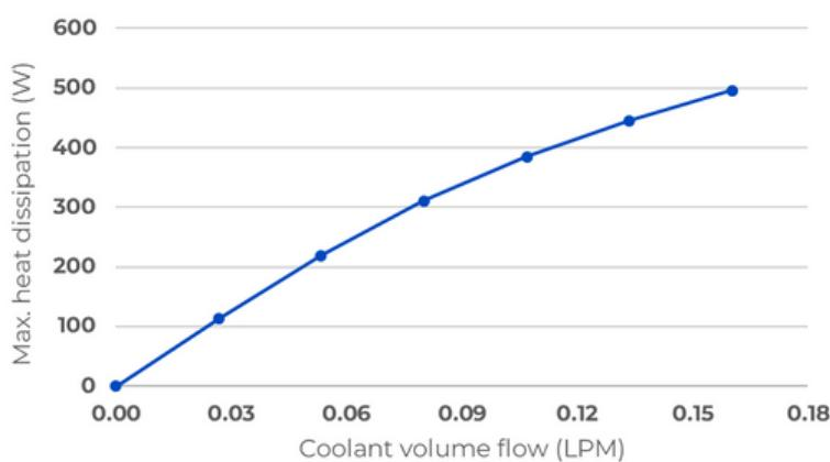
\*Heat dissipation considering 100°C fixed coil-former temperature.
