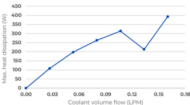
\*Heat dissipation considering 100°C fixed coil-former temperature.
