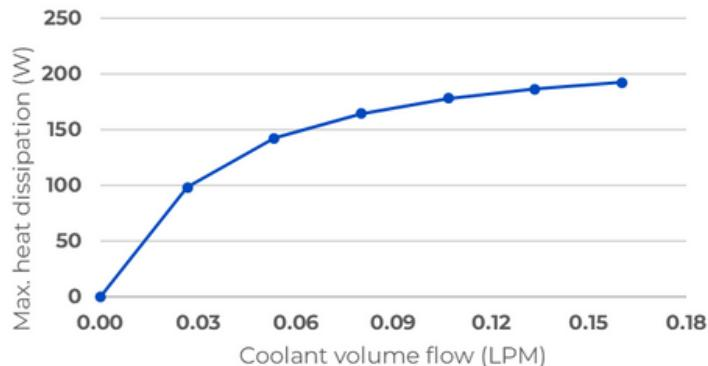
\*Heat dissipation considering 100°C fixed coil-former temperature.
