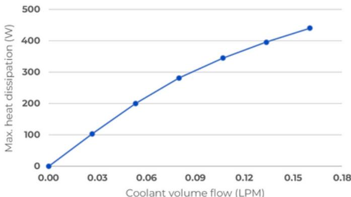
\*Heat dissipation considering 100°C fixed coil-former temperature.
