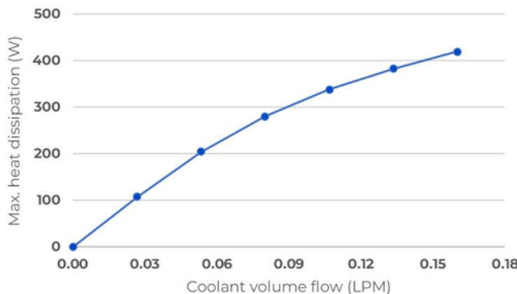
\*Heat dissipation considering 100°C fixed coil-former temperature.
