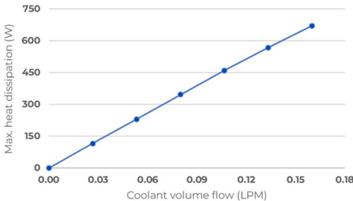
\*Heat dissipation considering 100°C fixed coil-former temperature.
